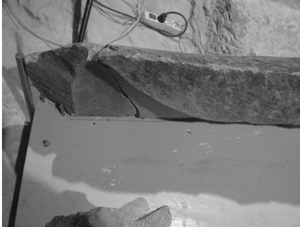
Fig. 9. Lower right side of lid with stainless steel dowels inserted to prevent slippage.
