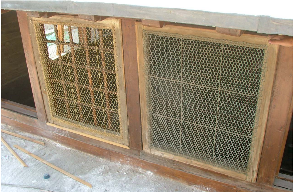
View of the samples of the steel mesh (on the left) and the one of the Comité (on the right)
